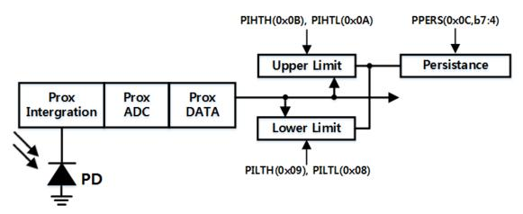
Figure 3. Programmable Interrupt
